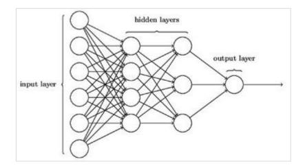
The layers between input and output are referred to as hidden layers, and the density and type of connections between layers is the configuration. For example, a fully connected configuration has all the neurons of layer L connected to those of L+1. For a more pronounced localization, we can connect only a local neighbourhood, say nine neurons, to the next layer. Figure 1-9 illustrates two hidden layers with dense connections.
